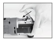
Close the latch and lock it into place. This will tighten the grip on the tool beyond-finger tight.
