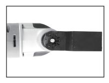
Ensure the pins on the tool holder align correctly with the holes in the tool.
