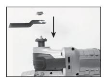
Place the desired tool into the tool holder paying attention to the direction in which the tool is pointing then replace the locking nut at finger-tightness.
