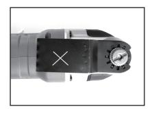
Never attach the blade with the cutting edge pointing backwards.
